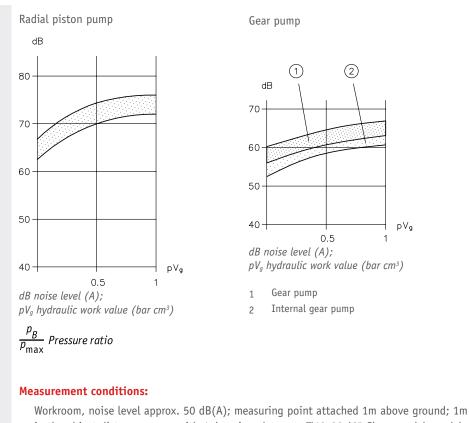
Workroom, noise level approx. 50 dB(A); measuring point attached 1m above ground; 1m in the object distance, pump with 4 damping elements Ø40x30 (65 Shore model, model damping element no. 20291/V).
