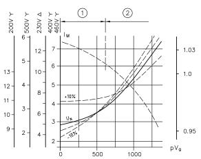
$I_M$  motor current (A);  $pV_g$  hydraulic work value (bar cm<sup>3</sup>);  $Q_{Pu}$  delivery flow curve (tendency) 1.0
