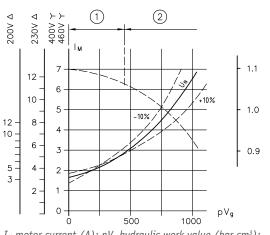
$I_M$  motor current (A);  $pV_g$  hydraulic work value (bar cm<sup>3</sup>);  $Q_{Pu}$  delivery flow curve (tendency) 1.0
